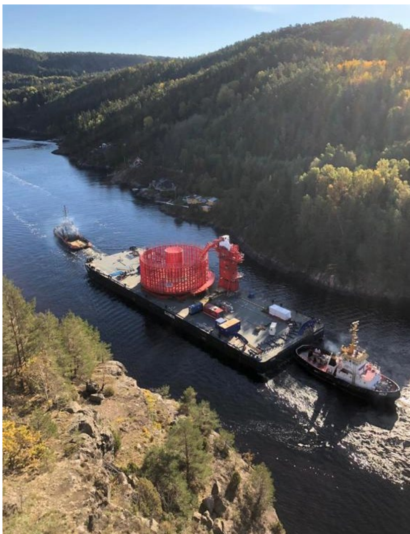
Figure 1 • Blue Offshore's BC01 23m OD, 10m fill height, mobilized on DAMEN TESS, in transit.
