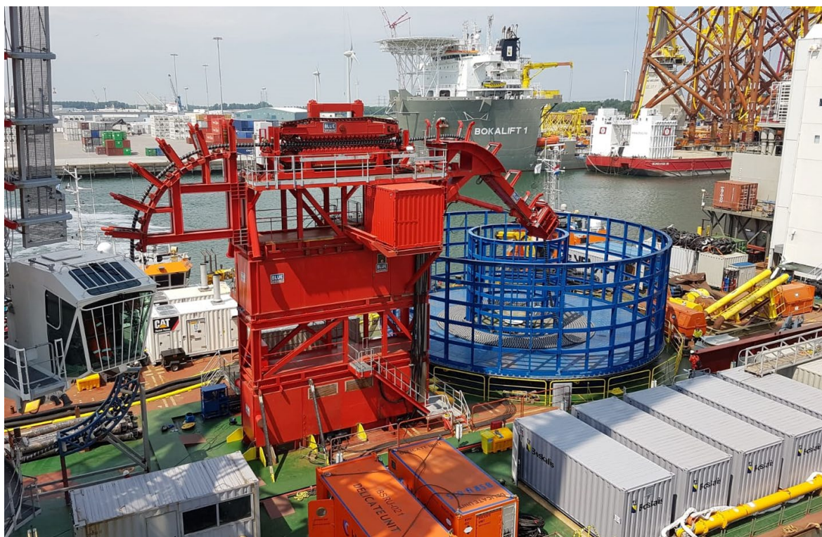
Figure 2 • Blue Offshore's loading tower on Boskalis' Giant 7, integrated with VBMS equipment.
