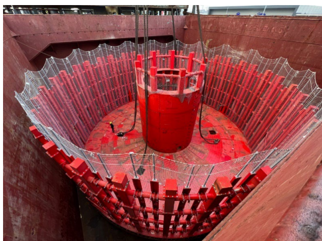
Figure 1&2 • One of our Basket Carousels positioned (during spooling operations) in the holds of the cargo vessel Edward Oldendorff.
