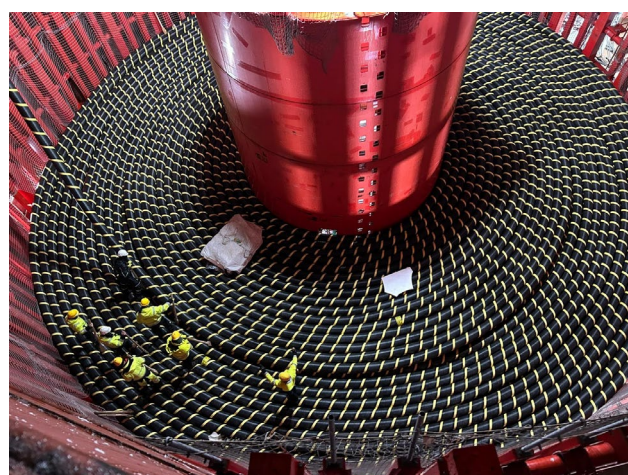
Figure 1&2 • One of our Basket Carousels positioned (during spooling operations) in the holds of the cargo vessel Edward Oldendorff.
