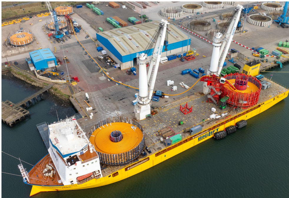
Figure 8 • Load-Out from Storage Tank to HLV
