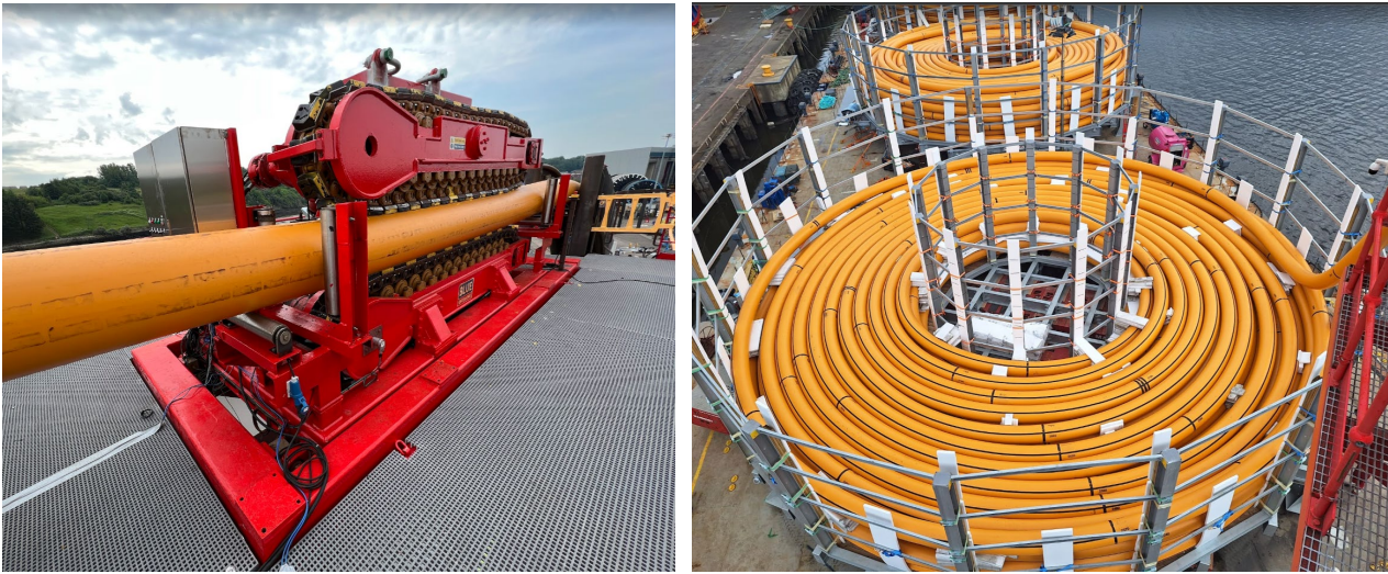
Figure 7 • Loading the flowlines into the tanks on the barge
