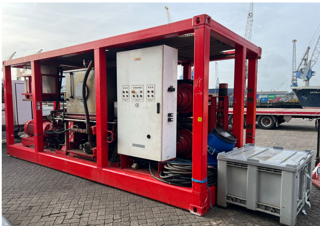
Figure 1 • Containerized 20'ft - 10Te Tensioner 02 with integrated HPU
