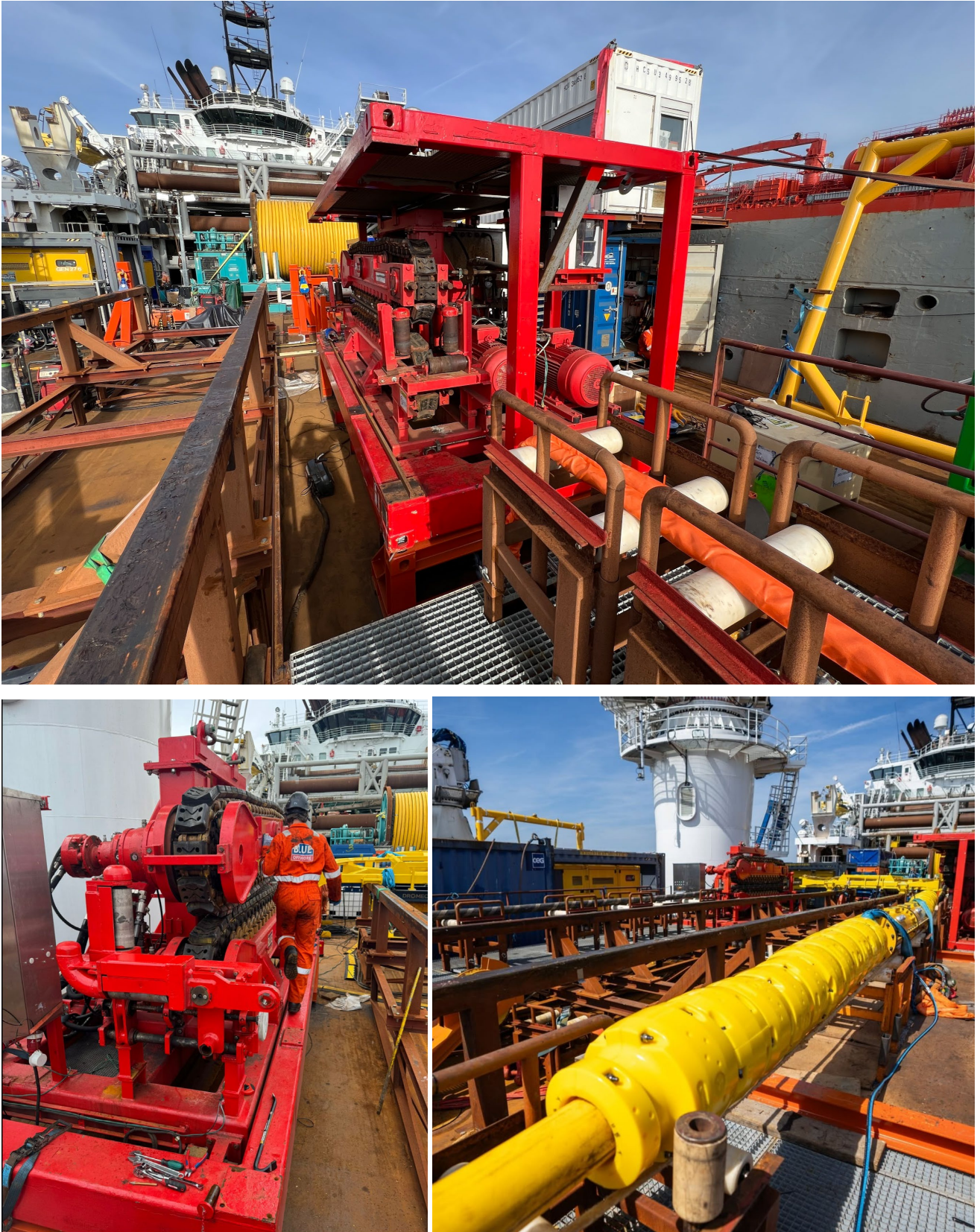
Figure 3 • 10Te Tensioner-02 & 15Te Tensioner-03 onboard Skandi Hera
